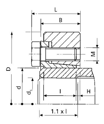
$\begin{array}{lll} \text{B mm} & = 58.0 \\ \text{d H8 mm} & = 140 \\ \text{D mm} & = 230.0 \\ \text{ds mm} & = 100 \\ \text{F kN torque} = 398 \\ \text{H} & = 7.0 \\ \text{I mm} & = 47.0 \\ \end{array}$
